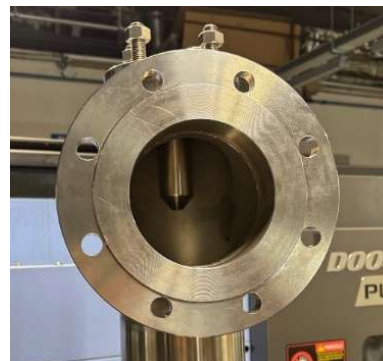
Spray nozzle section view
